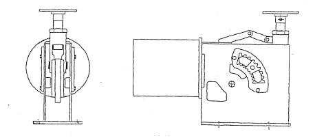
Connection to the pipe with load flange and pipe saddle EHS-4 (for example)
