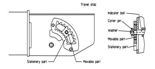
By turning the load column the movable part has to be positioned in the matching serrations until no further load is transferred to the stationary part of the travel stop, I. E. the movable part can be moved by hand at the indicator bolt.
